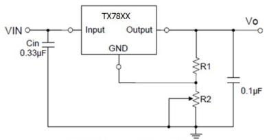
Fig.3 Adjustable Output Regulator
